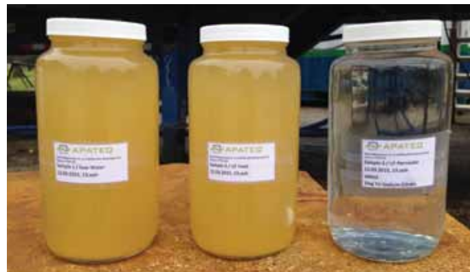
From left to right: produced water, water after primary treatment, clean water after ultrafiltration
